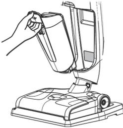
The type plate is located behind the dirt water tank. The dirt water tank needs to be removed to see the information on the type plate.
